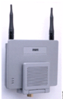
Figure 23 Cisco AP1200 Mounted to a Wall
