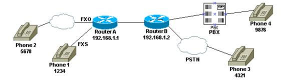
When a user picks up Phone 1 or when the PSTN number is dialed for the FXO line, the router provides the dial tone to the calling party (debug). The user then enters the digits and receives the dial tone from the terminating PBX/CO. The user then dials the destination number (9876 or 4321), and gets to the other phone. Make sure Router B does not send any digits to the PBX/CO.
