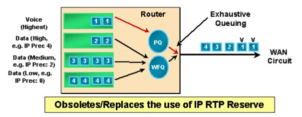
**Note:** IP RTP Priority allows bursting the PQ when there is available bandwidth on the default queue (WFQ). However, it strictly polices the PQ contents when there is congestion on the interface.
