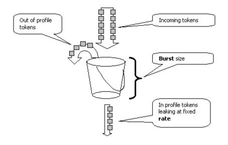
**Note:** The traffic is not buffered in the bucket, as it may appear in the image above. The actual traffic does not go through the bucket at all; the bucket is only used to decide whether the packet is in-profile or out-of-profile.
