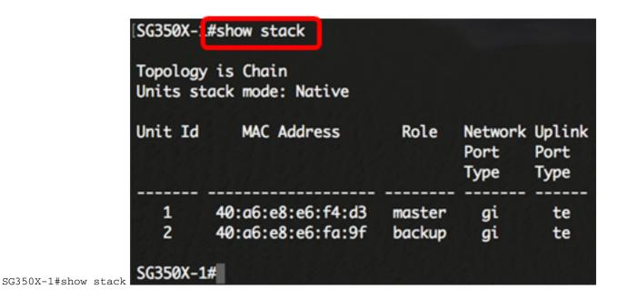
In this example, the configured unit 2 is now known as the Standby switch of the stack.
