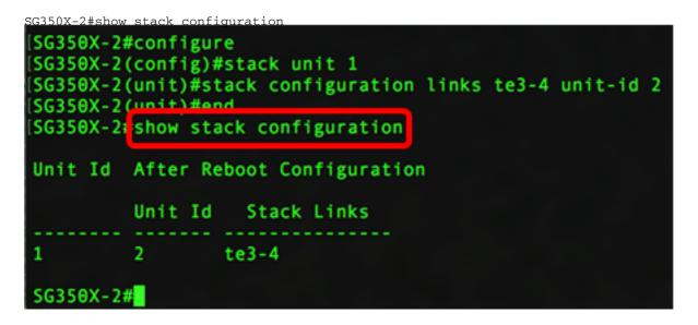
In this example, the Unit 2 switch now uses te3-4 as stack links. These settings will take effect after the switch reboots.
