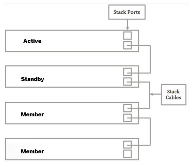
• Ring - Each unit is connected to the neighboring unit. The last unit is connected to the first unit. The image below shows a ring topology of a four-unit stack:
