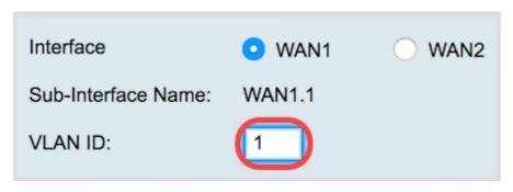
**Note:** The Sub-Interface Name area automatically updates based on the WAN and VLAN ID entered. In this example, WAN1.1 is displayed indicating WAN 1 and VLAN 1.
