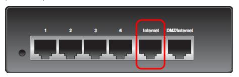
**Note:** The above image is the back of a RV042G VPN Router. All other routers listed under the applicable devices heading will look different, but still maintain the Internet and DMZ/Internet ports.
