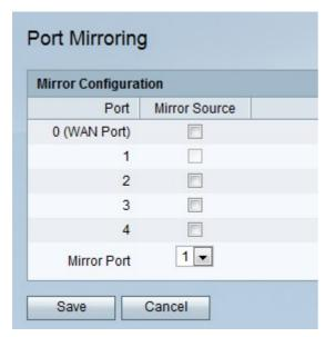
Step 2. Check the check boxes of the ports that will be mirrored from the *Mirror Source* column of the *Mirror Configuration* table.
