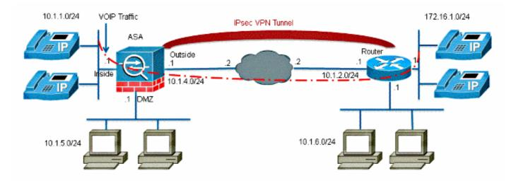
**Note**: Ensure that IP phones and hosts are placed in different segments (subnets). This is recommended for a good network design.
