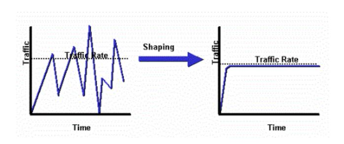
**Note**: Traffic shaping is only supported on ASA Versions 5505, 5510, 5520, 5540, and 5550. Multicore models (such as the 5500-X) do not support shaping.
