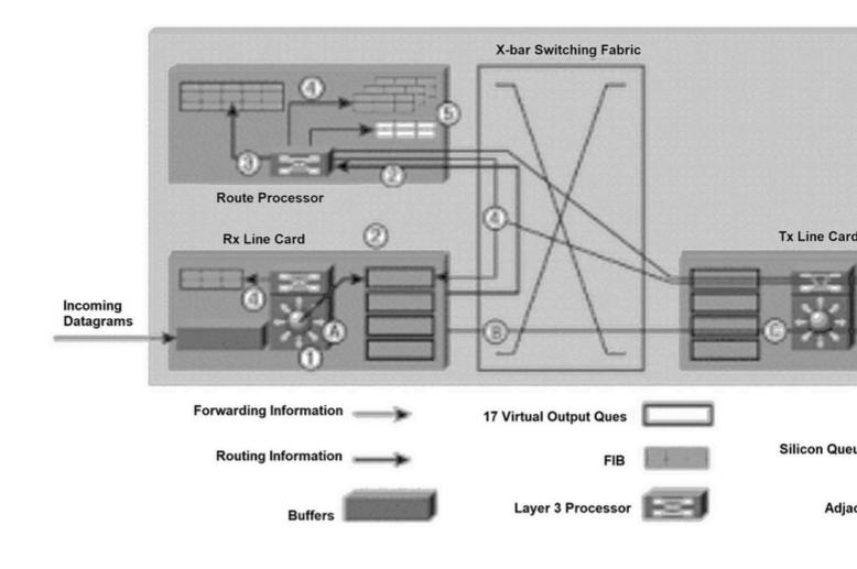
Path Determination and Layer 3 Switching Diagram
