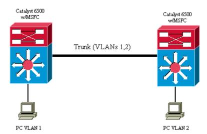
The diagram shown illustrates a physical topology of a typical Layer 3 (L3) network.
