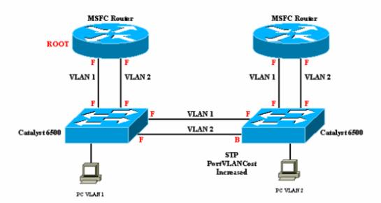
In this diagram, the MSFC blocks on the VLAN 2 connection to switch 2. The MSFC only blocks L2 frames from going out the VLAN 2 connection to the switch and not L3 frames. This is because the MSFC is a L3 device that is able to determine the difference between a frame that needs to be bridged or routed. In this example, there is no network segmentation, and all network traffic flows as desired. Although there is no network segmentation, there is still one single instance of STP for all VLANs.
