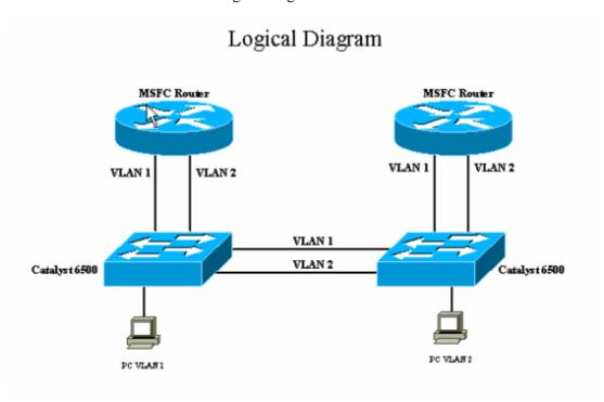
Once the Multilayer Switch Feature Cards (MSFCs) in both Catalyst 6500 are configured for bridging with the IEEE STP, both VLAN 1 and VLAN 2 are bridged together in order to form one single instance of STP. This single instance of STP contains only one STP root. Another way to view the network with the MSFC's bridging is to consider the MSFCs as separate bridges. One instance of STP that involves the MSFCs can result in an undesirable network topology.
