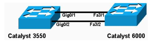
**Note:** The Gigabit Ethernet interface on the Catalyst 3550 is a 10/100/1000 Mbps negotiated Ethernet interface. The Gigabit port on the Catalyst 3550 can also be connected to a FastEthernet (100 Mbps) port on a Catalyst 6500/6000.
