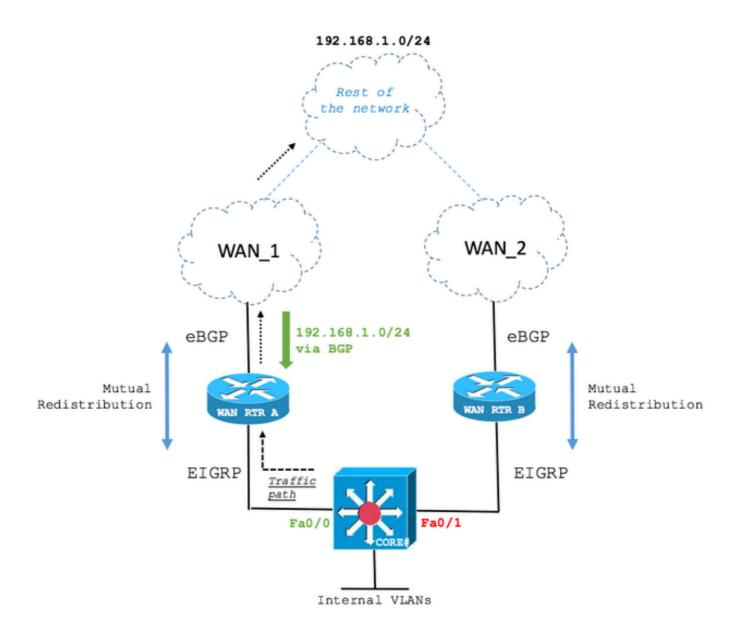
The CORE Layer 3 Switch receives the 192.168.1.0/24 route via EIGRP from WAN RTR A and WAN RTR B. The path over WAN RTR A is elected.
