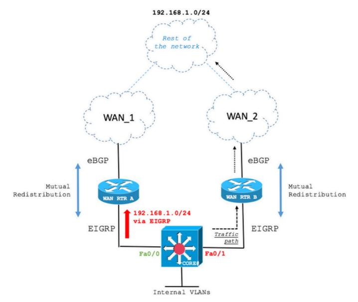
The primary WAN link has been restored. However, the CORE Switch still routes over the backup path as seen on the next output:
