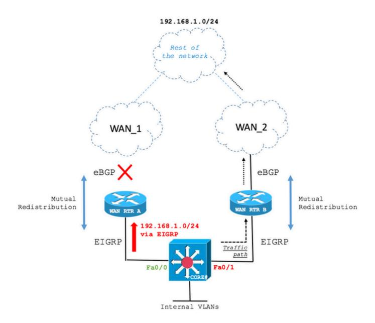
In case of a link failure, the CORE Switch now installs the route via the second best EIGRP path which is WAN RTR B.
