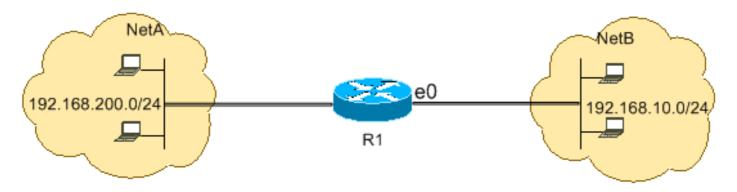
This configuration allows the IP packets with an IP header that has a source address in the network 192.168.10.0/24 and a destination address in the network 192.168.200.0/24 access to NetA. There is the implicit deny all clause at the end of the ACL which denies all other traffic passage through Ethernet 0
