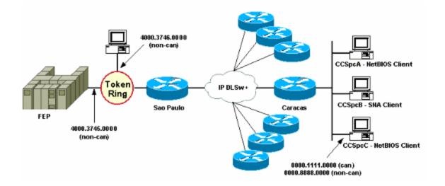
In this example, a new SNA device (4000.3746.0000) is added at the Sao Paulo location. This machine needs to establish communication with a device at another location (peer 3.3.3.1). The Sao Paulo router runs this configuration.
