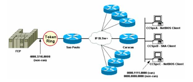
In the network diagram, a data center router (Sao Paulo) is depicted with a connection to the mainframe. This router receives multiple DLSw+ peer connections from all the remote branches. Each remote branch has both Systems Network Architecture (SNA) and NetBIOS clients. There are no NetBIOS servers in the data center that need to get accessed from the remote offices.
