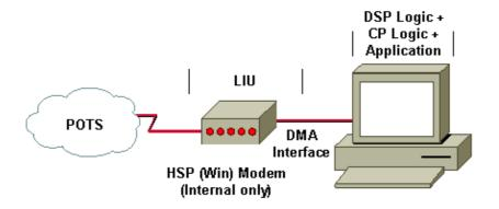
In HSP modems, the modem itself only consists of the LIU. It shunts the PCM–encoded waveform through the internal bus to the CPU of the host computer emulating the DSP.
