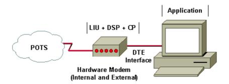
In a hardware modem, the modem handles LIU, DSP and CP functions. Hardware modems have historically been the best modems performance–wise, and also the most reliable type. Hardware modems can be external or internal. With external modems, a physical cable (such as an RS–232 serial interface) connects the computer to the modem. In internal hardware modems, the internal bus of the computer handles this function.
