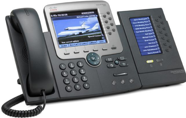
Figure 3. Cisco Unified IP Phone 7975G with Two Cisco Unified IP Phone Expansion Module 7916 Modules
