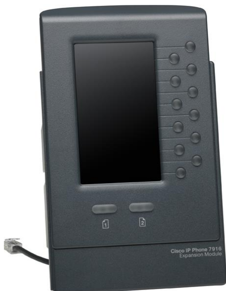
Figure 1. Cisco Unified IP Phone Expansion Module 7916
