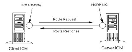
The ICM-to-ICM link shown in Figure 1-2 is a connection in one direction only. It allows the Client ICM to send route requests to the Server ICM, but not the other way around. It is possible to additionally reverse the roles of the ICMs as well, so that each ICM can send route requests to each other. In this case, each ICM needs to be configured for an ICM Gateway and an INCRP NIC, as shown in Figure 1-3.
