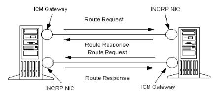
INCRP supports direct connections between two ICMs only. ICMs that are not directly connected with an ICM-to-ICM link cannot send each other route requests through another ICM.
