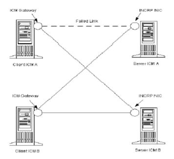
• If an INCRP NIC fails, the Client ICM's routers are synchronized and can communicate via the remaining INCRP NIC.
