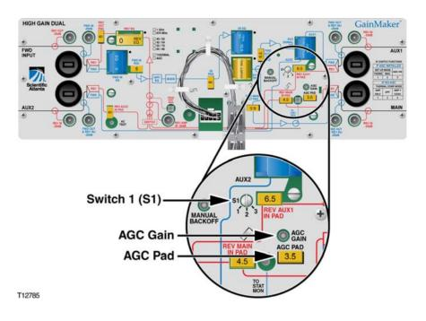
3 Remove the original (standard) AGC module.Note: Pull straight up on the module housing to remove the module.
