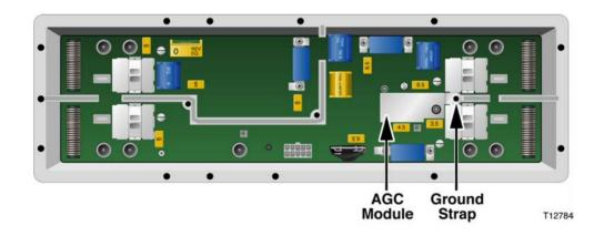
4 Install the QAM AGC module.
