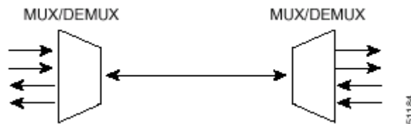
Figure C-17: Multiplexing and Demultiplexing in a Bi-Directional System
