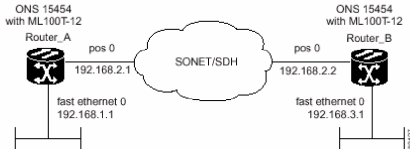
Figure 5-23: ML-Series Card-to-ML-Series Card POS Configuration
