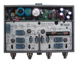
Settings for the EGC amplifier can be established or modified using a handheld programmer terminal. Settings from one amplifier can be uploaded to the handheld programmer terminal for downloading to other amplifiers in order to streamline their configuration. Different forward gain settings can be obtained in the amplifier, enabling it to support several different applications within the network allowing a single amplifier model to help reduce inventory and lower costs.
